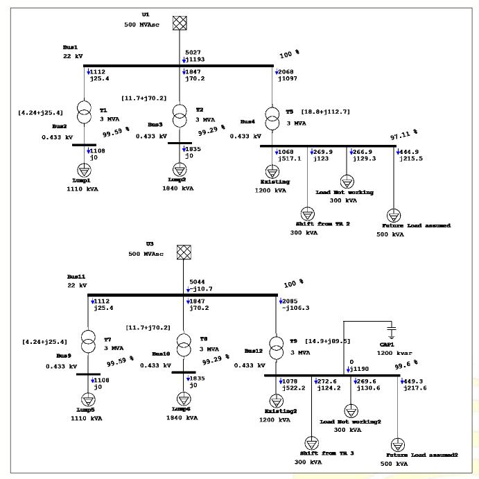
Branch losses with and without correction in exact numbers will be as shown above. Loss in TR 5 will reduce from 18.8KW to 14.9KW if power factor is corrected. TR5 secondary bus voltage will improve from 97.11% to 99.6%. These accurate calculations help in assessing the payback period.
